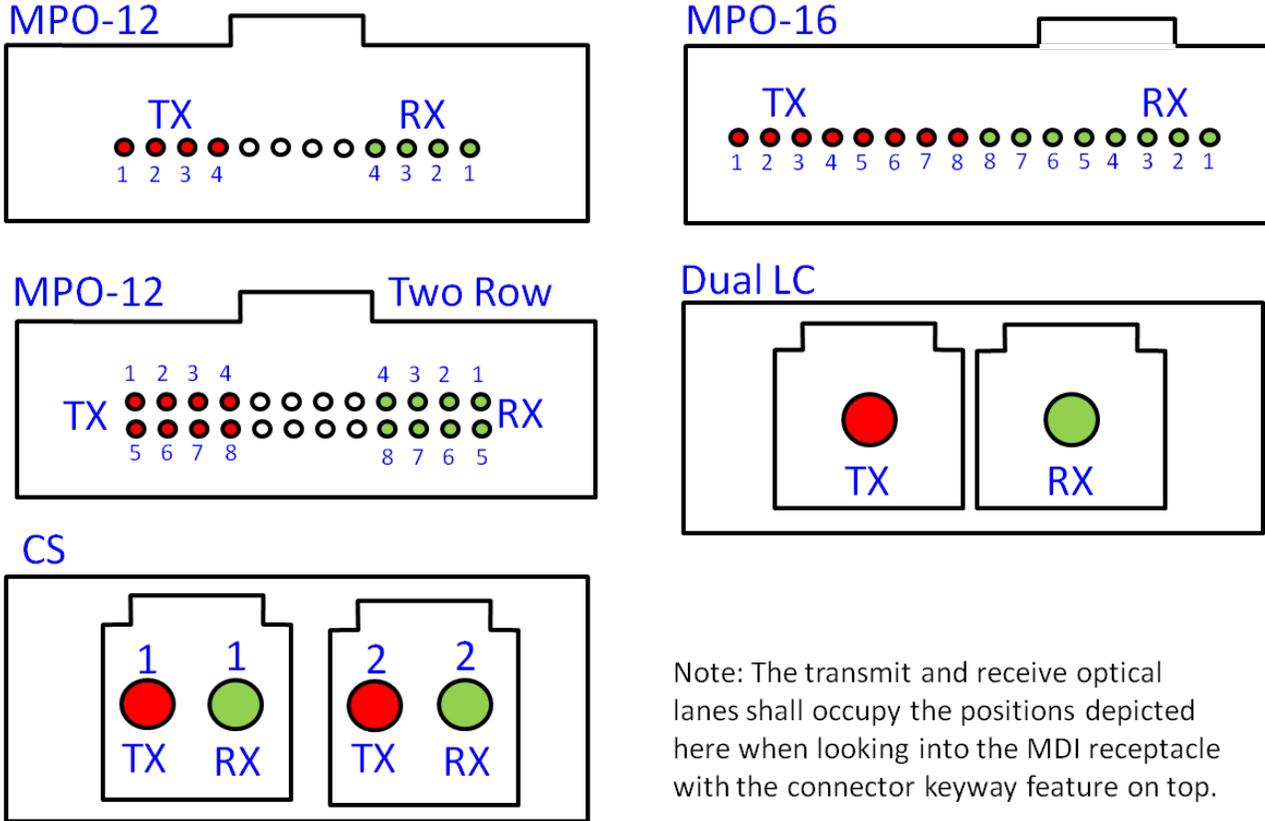
Figure 31: Optical Media Dependent Interface port assignments
