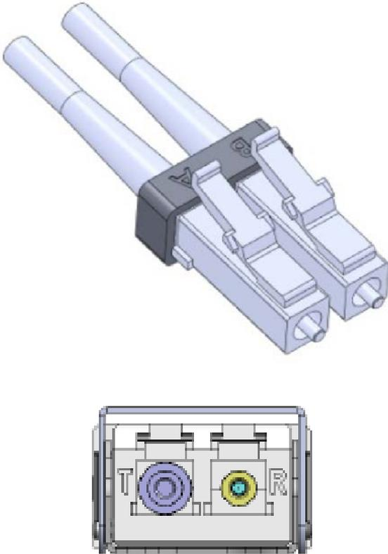
**Figure 35: Dual LC optical patchcord and module receptacle**
