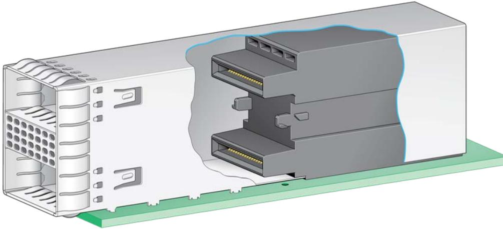
**Figure 18: Integrated connector in 2x1 stacked cage**
