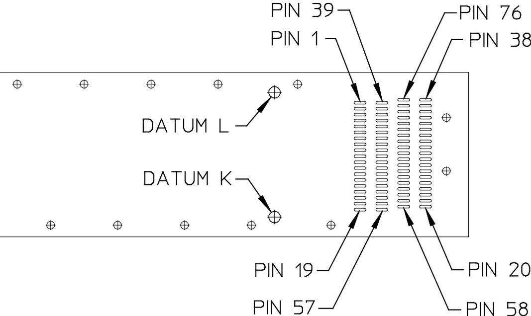
Figure 30: SMT Connector and Host PCB Pin Numbers
