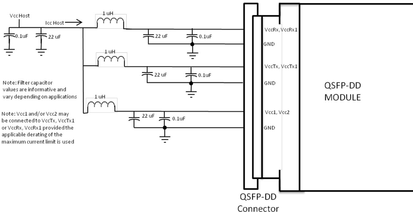
**Figure 6: Recommended Host Board Power Supply Filtering**
