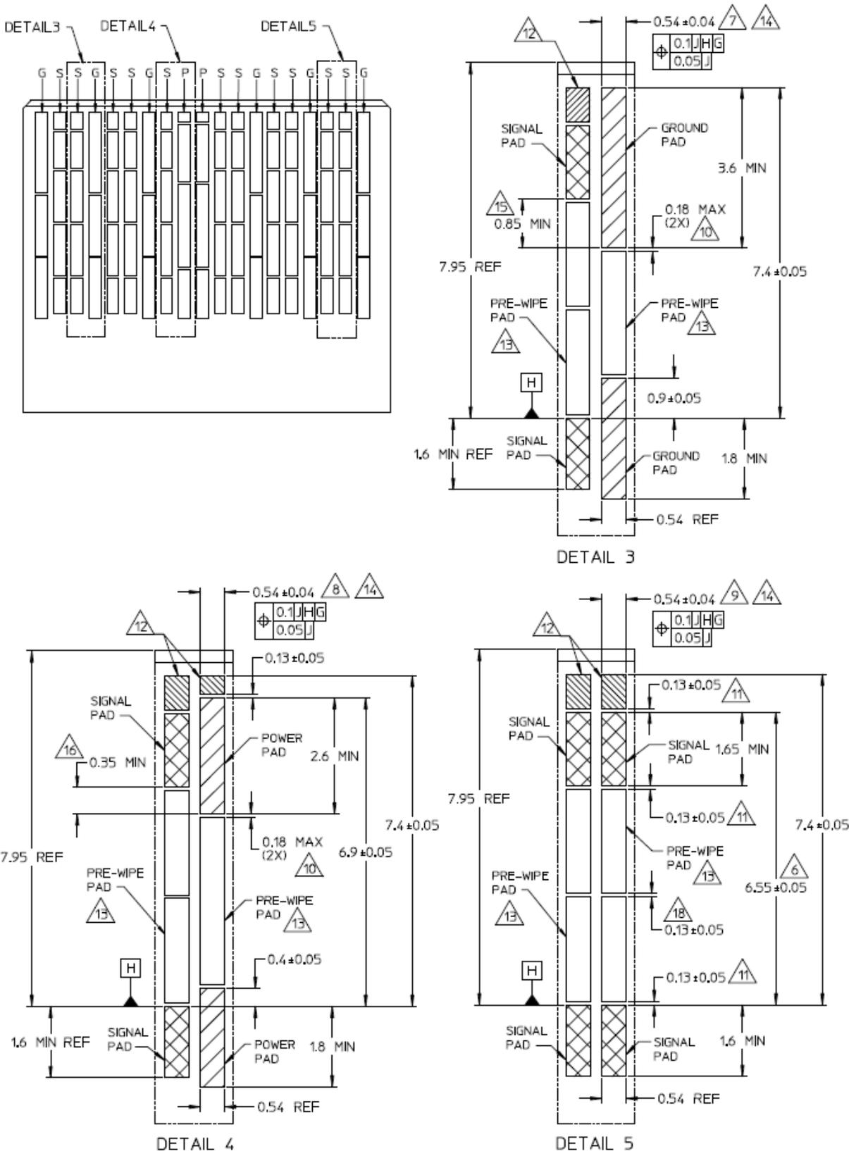
Figure 17: Module pad dimensions
