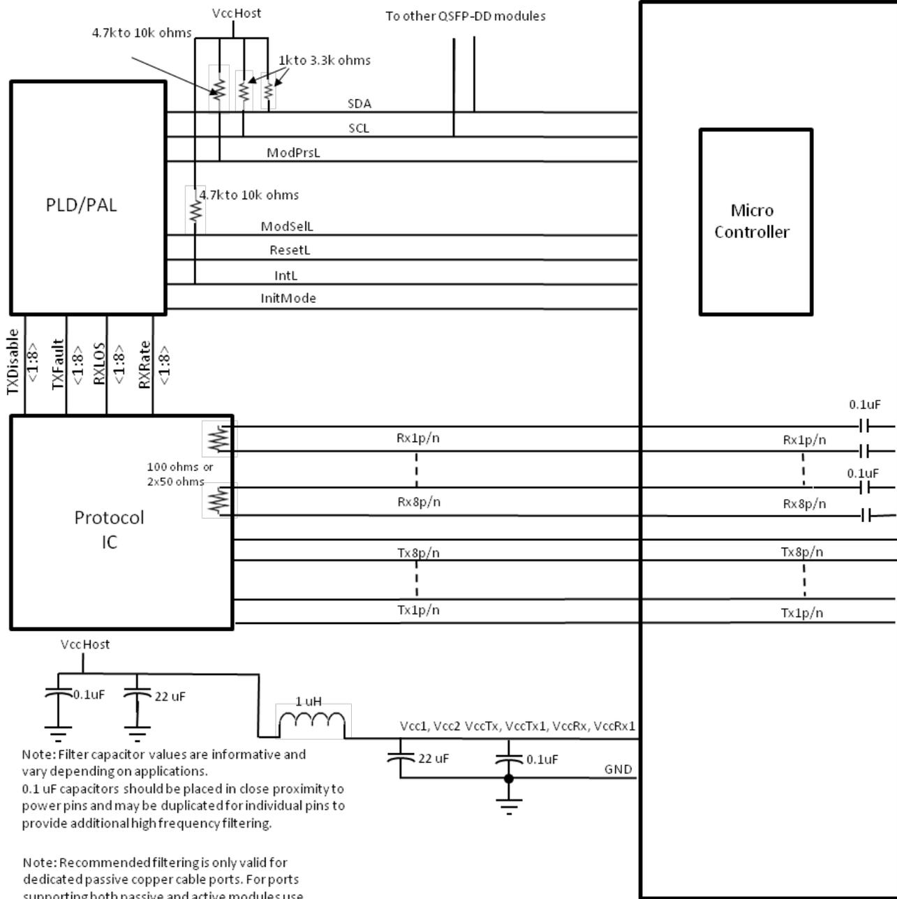
Note: Filter capacitor values are informative and vary depending on applications. 0.1 uF capacitors should be placed in close proximity to power pins and may be duplicated for individual pins to provide additional high frequency filtering.
